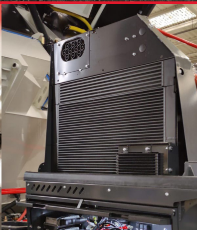
Combi cooler radiator Single triple stack cooling pack for improved cooling performance and ease of cleaning.
